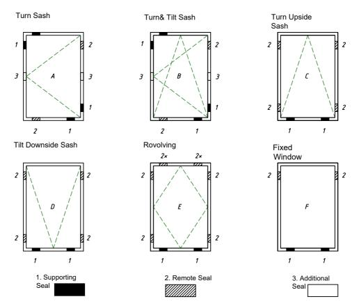
Supporting Seal-in Case Of Revolving Sash
